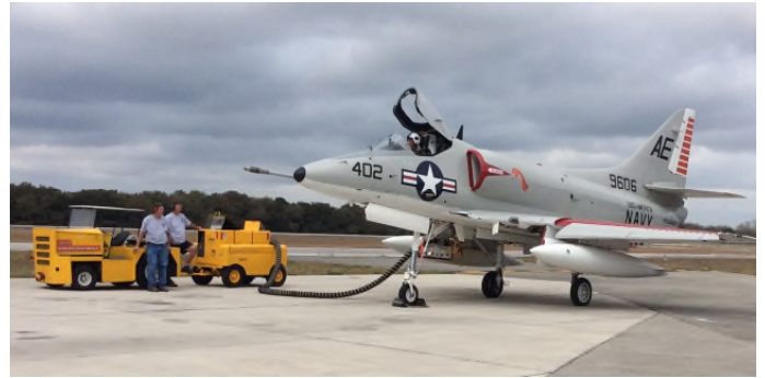
A-4C Skyhawk , getting ready to start, is shown here with its auxiliary power unit.
